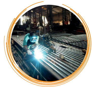
Water Wall Panel Manufacturing
