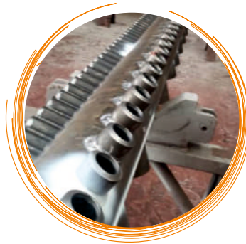
Boiler Header Manufacturing
