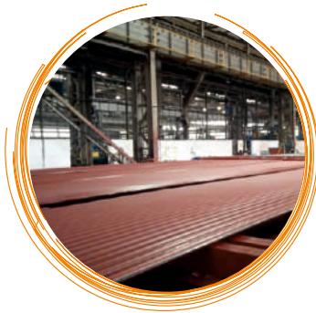
Water Wall Panel Manufacturing
